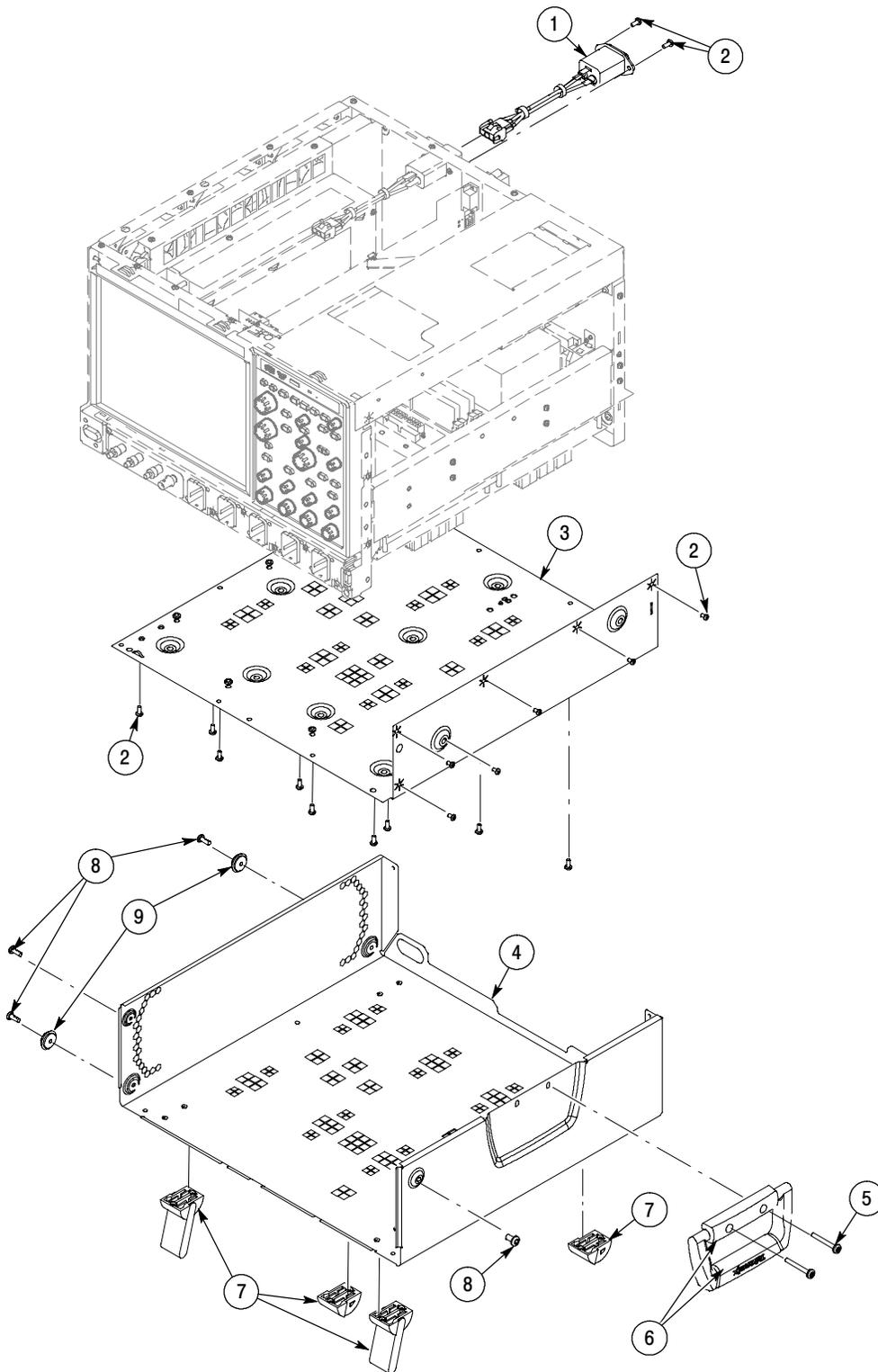
Figure 5-8: External parts 2 ( $\geq 4.0$  GHz models)
