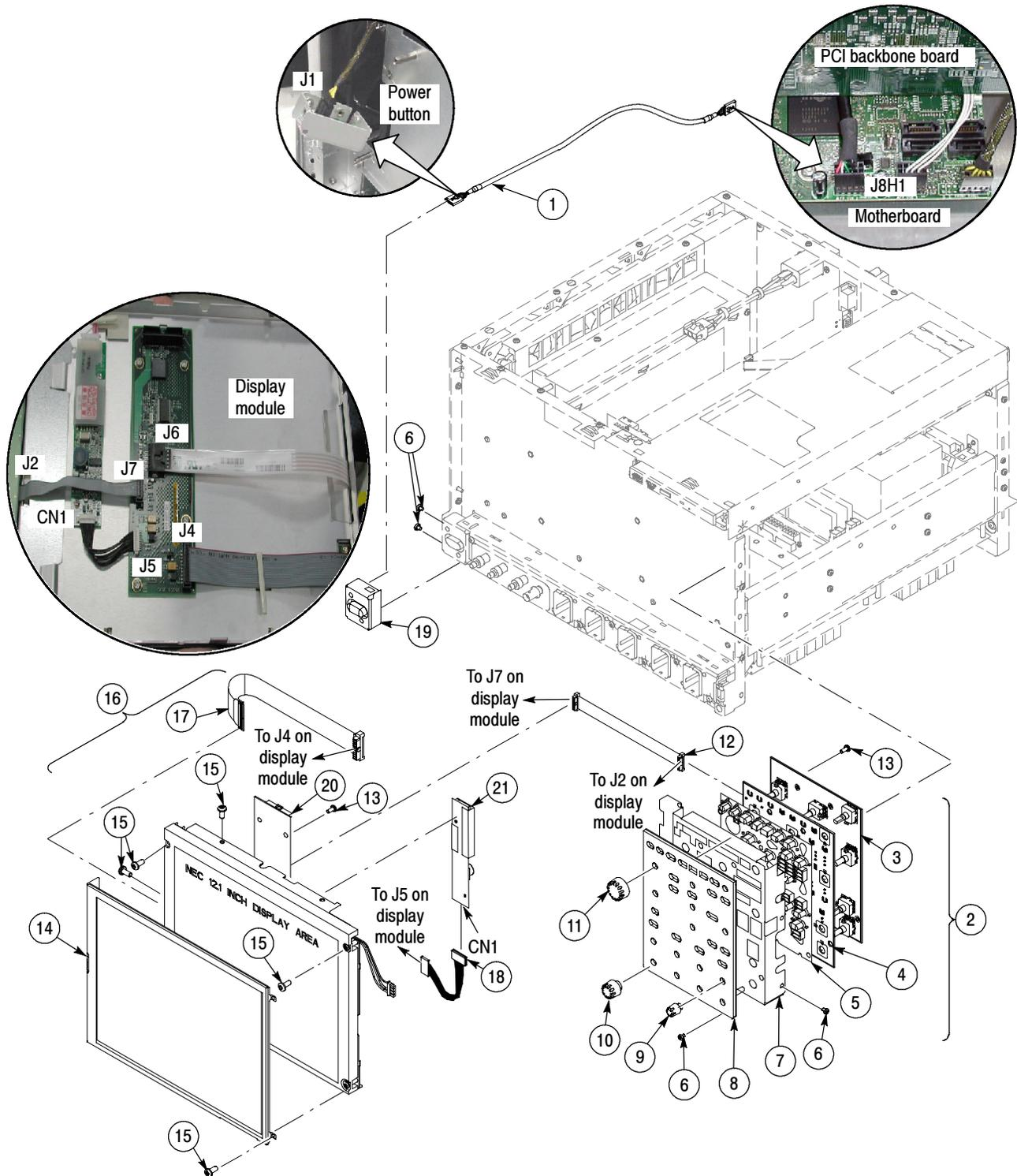
Figure 5-9: Front panel and display ( $\geq 4.0$  GHz models)
