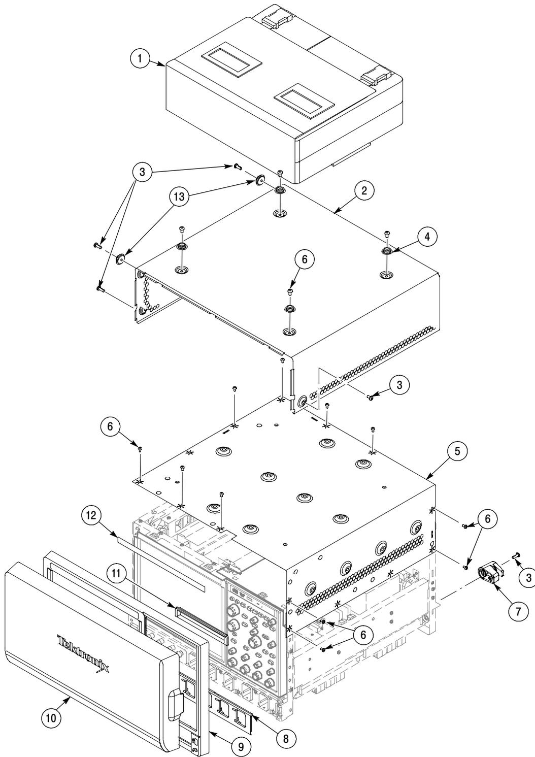
Figure 5-7: External parts 1 ( $\geq 4.0$  GHz models)
