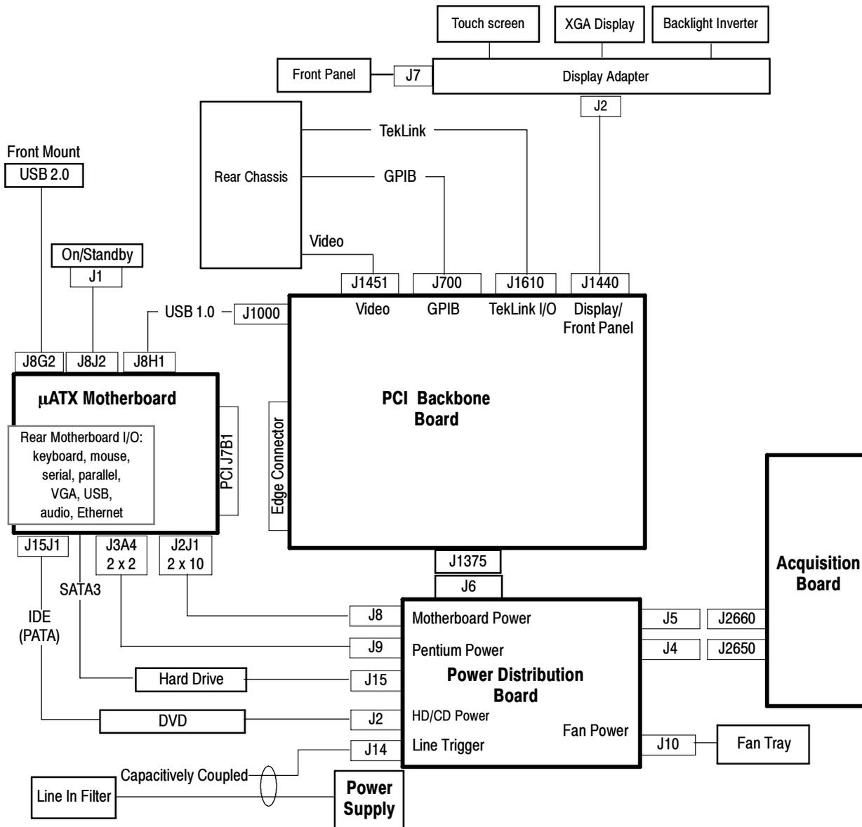
Figure 2-2: DPO70000 and DSA70000 Series block diagram
