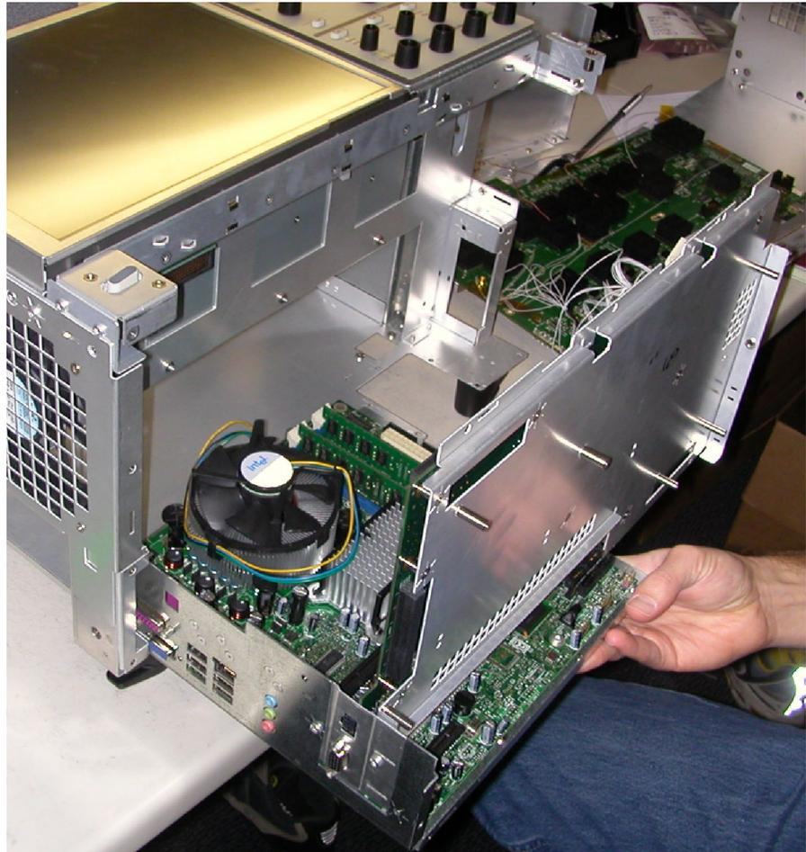
**Figure 4-3: Removing the  $\mu$ ATX/Power Interface assembly**
