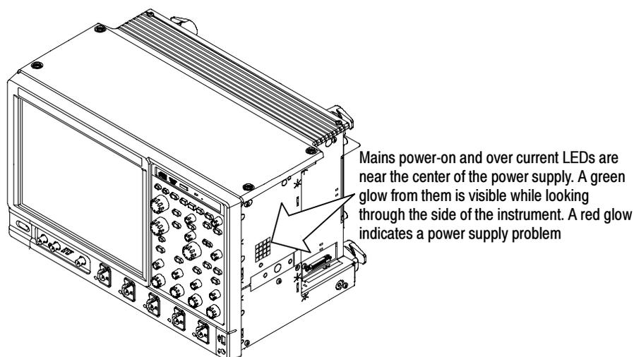
**Figure 4-5: Location of power-on and over current LEDs**
