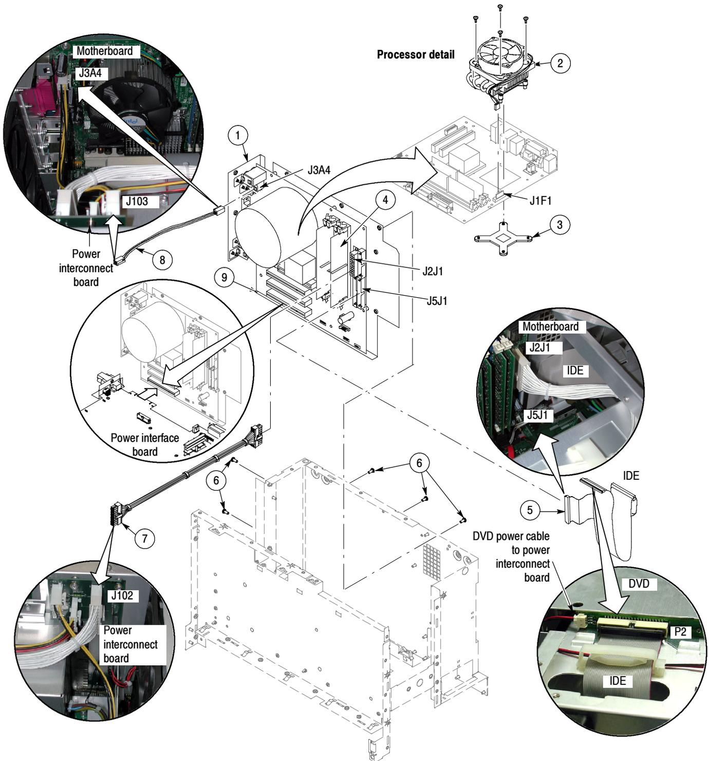
Figure 5- 4:  $\mu$ ATX Motherboard (<4.0 GHz models)
