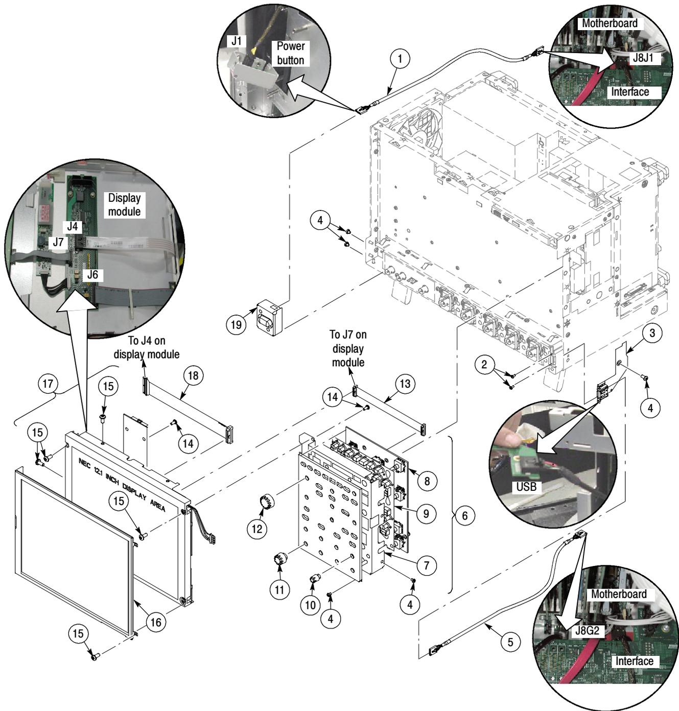
Figure 5-2: Front panel and display (<4.0 GHz models)
