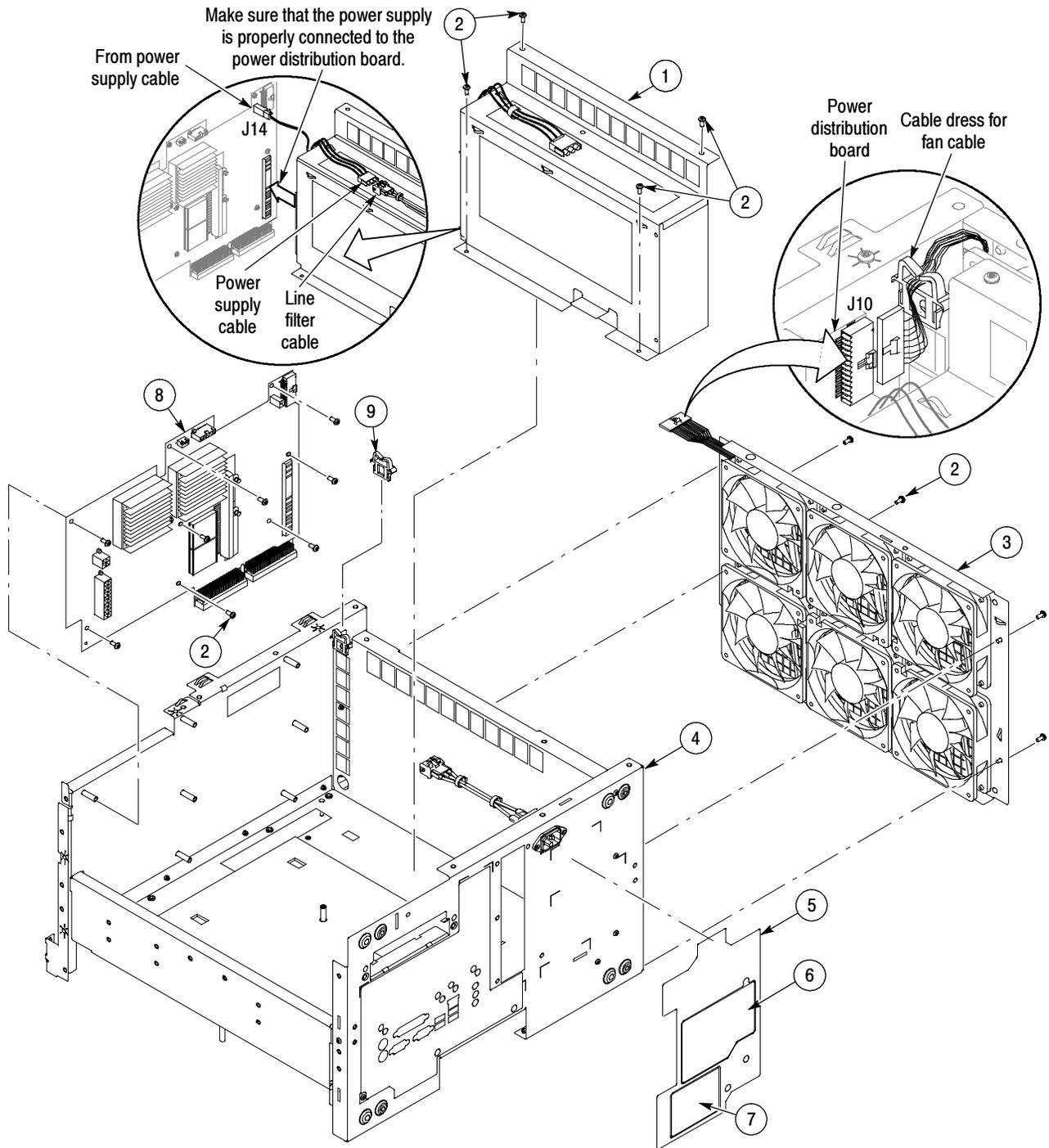
Figure 5-10: Power supply and fans ( $\geq 4.0$  GHz models)
