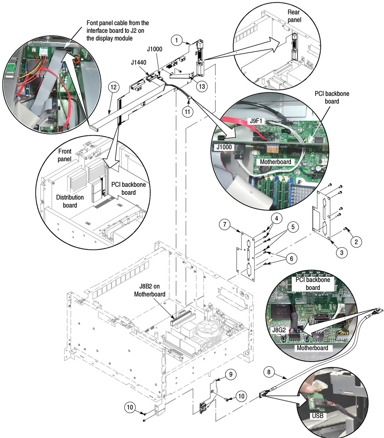
Figure 5- 13: Interface board (≥ 4.0 GHz models)
