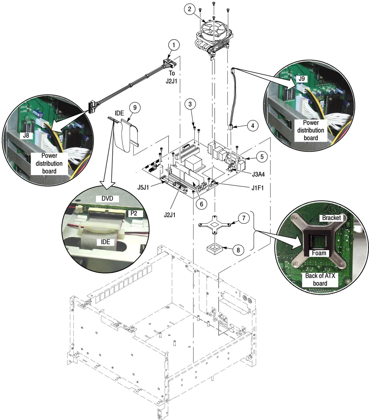
Figure 5-11: Atx assembly ( $\geq 4.0$  GHz models)
