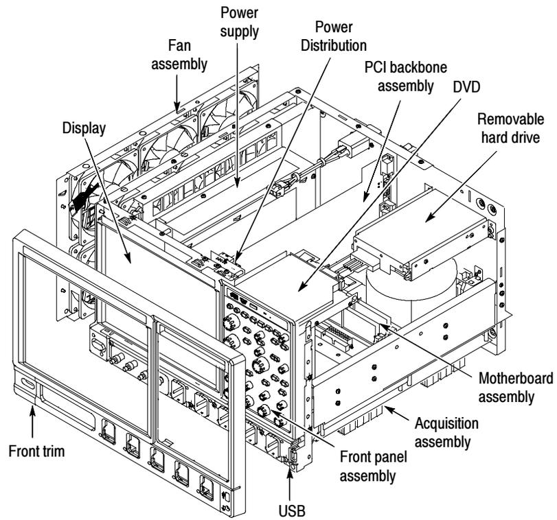
**Figure 4- 2: DPO7000 and DSA7000 Series module locations**
