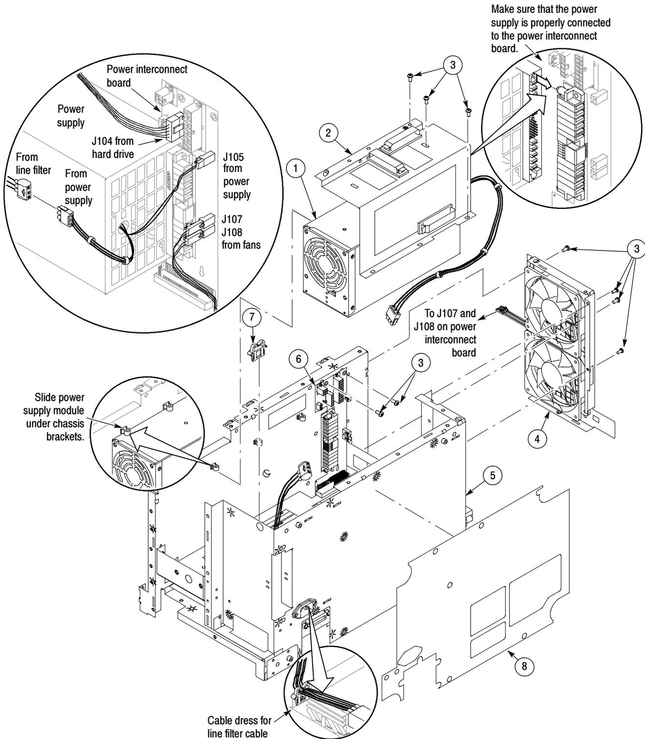
Figure 5-3: Power supply and fans (<4.0 GHz models)
