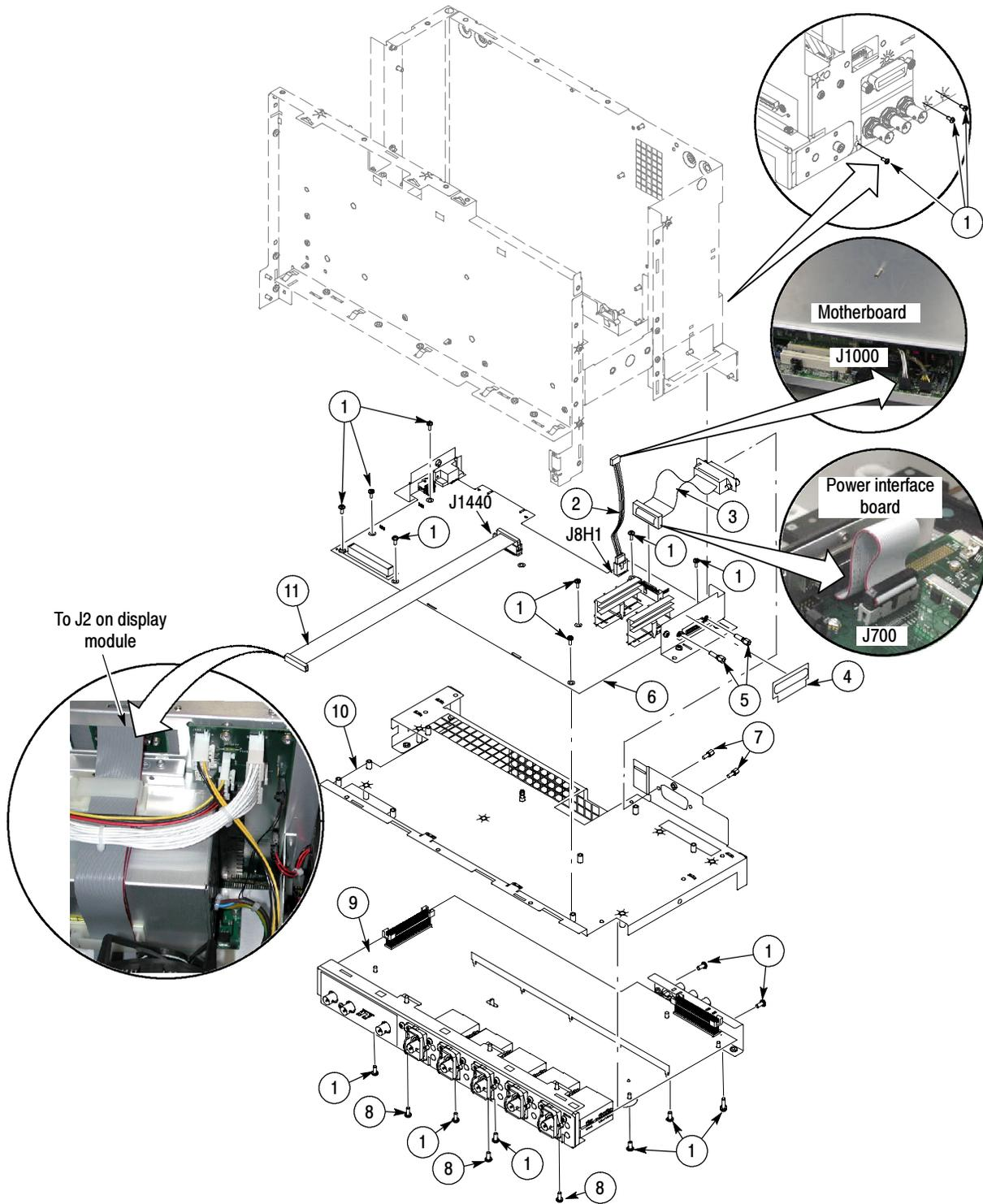
Figure 5- 5: Power interface and Acquisition assemblies (<4.0 GHz models)
